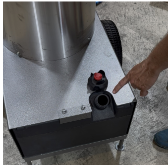
FUEL FILL PORT, FRONT OF UNIT
